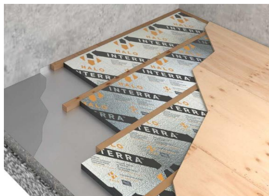
Figure 9. Insulation of Concrete Floor (Image from https://buildwithhalo.com/ )
